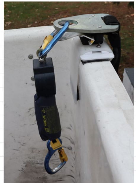
Figure 1: Never leave the safety lanyard attached to the Fasten Tracker detector!
